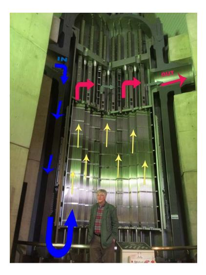
**Figure 2** illustrates how missing or damaged baffle bolts can cause the reactor to overheat. If the bolts fail, the plates will open, allowing the cooling water to deviate from its normally tightly constrained path through the reactor, risking overheating of the reactor core and an uncontrollable nuclear reaction and meltdown.
